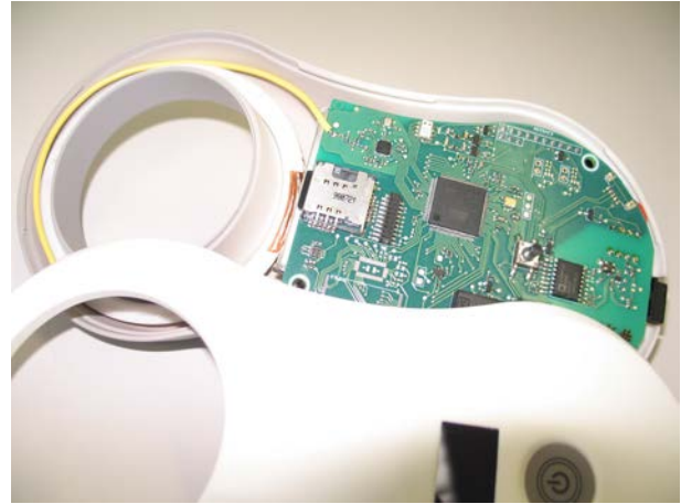
Atmel SAM7X in a battery powered charging and control system for a human medical implant Art of Technology AG for Sequana Medical AG (formerly NovaShunt AG)
